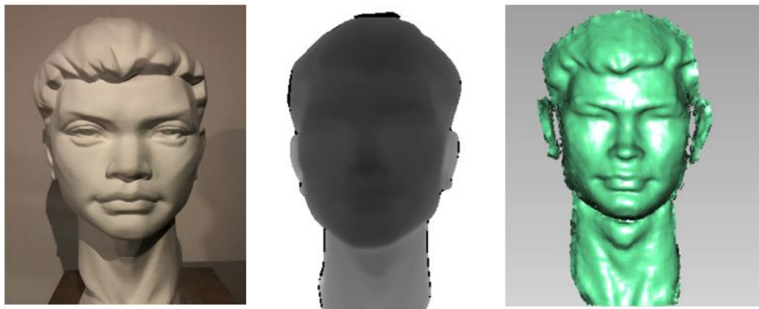
From left to right: original target, IR depth map, 3D point cloud generated from IR depth
